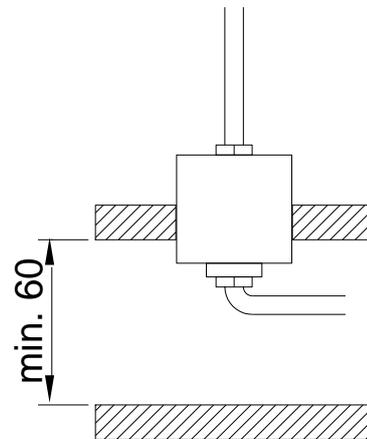
4. Insert the luminaire into the cutout and check if it works correctly.
